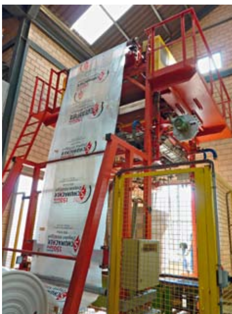
»11 The pallets full of bricks are shrink-wrapped in a Keller-built thigh-packer
